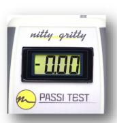
Passi Test is a tool designed for those who need to know exactly the real quality of the stainless steel. It consists of a "probe pen" – which will be put on the superface to be tested – containing the electrochemical system and a reading external unity.
